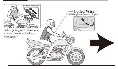
The Hit-Air (Shock-buffering Protection System) is to be worn as an outerwear when riding a motorcycle.
