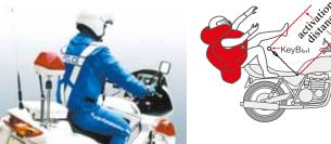
In a fall or crash, the shock-buffering protection system will be activated instantly after the distance from the rider to the motorcycle exceeds the "activation distance", when the key ball is pulled out of the key box to release CO2 gas into the neck, back. chest, side and hip airbags to inflate them and to absorb the impact on rider's body.
